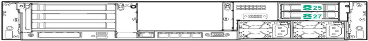
4DW chassis with 8 SFF drive cage
