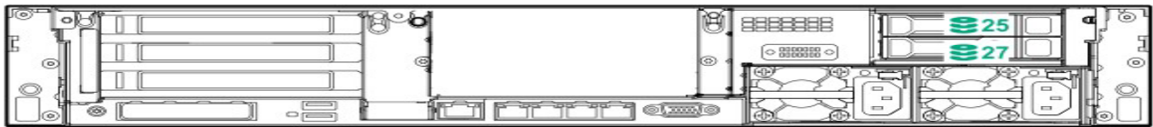
4DW chassis with 8 EDSFF drive cage
