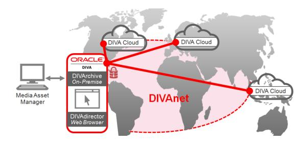
Customer site connectivity relies on the DIVAnet software and wide-area network (WAN) transfer acceleration software both provided by Oracle. The acceleration software also creates AES encrypted tunnels for a secure transfer of data from customer sites to DIVA Cloud sites.
