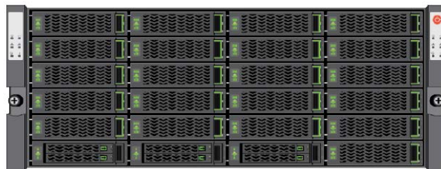
HPE Nimble Storage SF100/SF300 Secondary Flash Array (Base array, 4U; 21 bays hold carriers with Large Form Factor HDDs, 3 bays hold Dual Flash Carriers with Small Form Factor SSDs)
